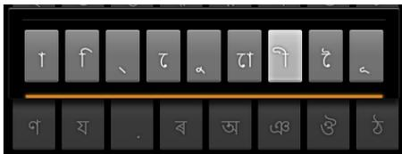
Fig. 15. The diacritic pop-up menu. The menu appears when a consonant key is held down.
