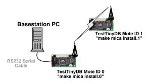
Figure 1: Two TinyDB motes set up to run a query.
