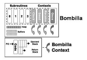
Figure 1: Bombilla Architecture and Execution Model: Capsules, Contexts, and Stacks
