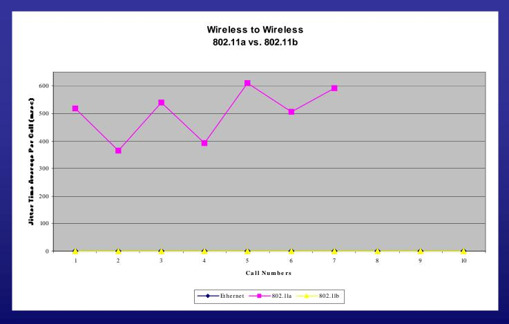
Each client's distance from AP ~15-20 ft. Peer-to-peer ~30-40 ft. Poor signal strength for 802.11a, excellent for 802.11b.
