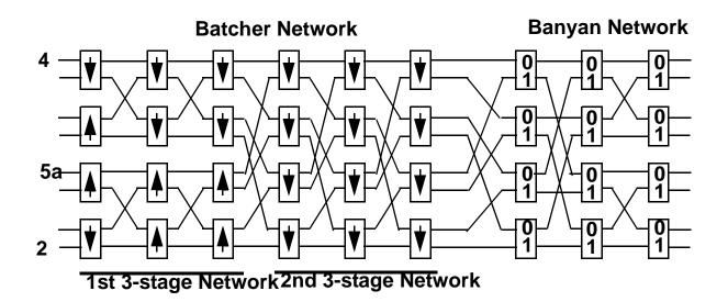
the 2x2 switch configurations (cross-over, or straight through) along their routes to destination ports.
