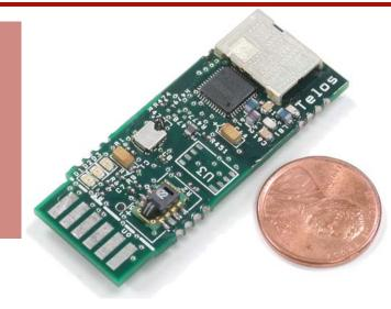
Designed at the University of California, Berkeley, by TinyOS developers, the Telos platform offers seamless vertical integration between the hardware and the TinyOS operating system. TinyOS is a small, open-source, component-based operating system also developed at UC Berkeley. TinyOS was specifically designed to support the networked sensor regime. By leveraging their intimate knowledge of both the hardware and TinyOS layers, Moteiv can promise the highest levels of support to their customers.
