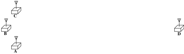
Figure 3: Situation where there is a candidate station B for an intermediate hop between A and C. Routes are chosen so as to minimize each packet’s total contribution to interference at distant stations (e.g. D).
