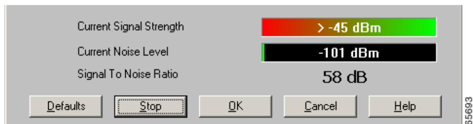
Figure 7-8 Bottom of Linktest Screen (with Test Running and Signal Strength in dBm)
