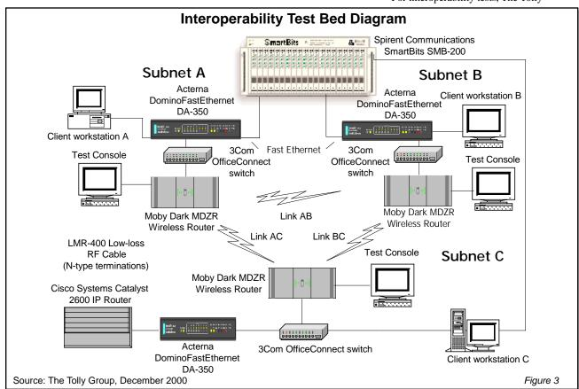
Group engineers used three Moby Dark Inc. MDZR Wireless Routers all running MobyBSD v. 0.34 and Moby Dark Router Traffic Controller (MRTC) v. 0.07. Each device had two 2.4-GHz ports equipped with Lucent WaveLAN Wireless Adapters and one 100Base-TX Fast Ethernet port. These devices were interconnected via RF (radio frequency) cable between the wireless ports. These ports had N type connectors and were linked by the use of miniature flat panel antennas with 6dBi gain.
