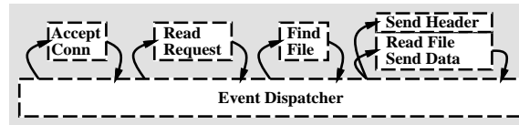
Figure 4.4 : Single Process Event Driven - The SPED model uses a single process to perform all client processing and disk activity in an event-driven manner.
