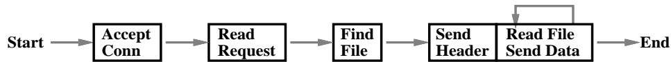
Figure 4.1 : Simplified Request Processing Steps - The minimum processing necessary for handling a single request for a regular file (static content) is shown in this figure.
